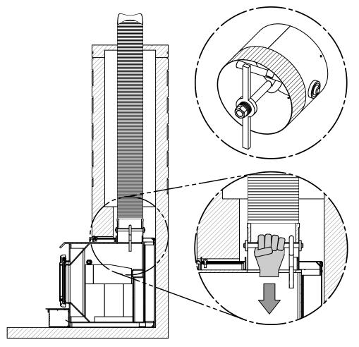
Figure 8: Liner fastening system
