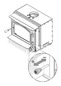
Figure 1: Air Intake Control
