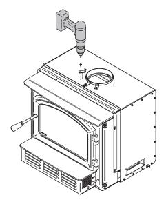
Figure 7: Securing the brackets
