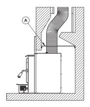
Figure 4: Block-off Plate
