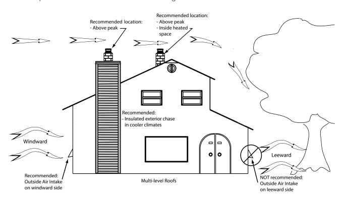
Figure 10: Air supply in conventional houses
