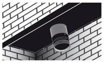
Figure 5: Block-off Plate
