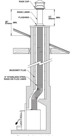
Figure 6: Liner Installation
